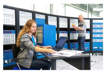
electronic devices (e.g. VSC bridges with PWM switching). The hardware is bundled into modular units called racks that allow easy expansion of the simulator's computing capability as required. With the fast computational speed of the RTDS hardware, analytical studies can be performed much faster than EMTP-type simulation programs.
