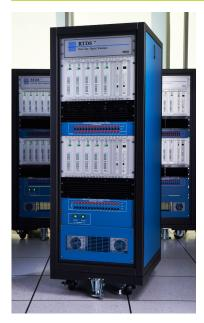
The parallel processing required by the RTDS Simulator is carried out by processor cards. These cards are mounted in card cages, known as racks, which are housed in cubicles. Different cubicle sizes are available to meet the varying simulation requirements of our customers. As the simulation demands of a user increases, processor cards can be added to the racks. As racks are filled, more cubicles can be acquired,
